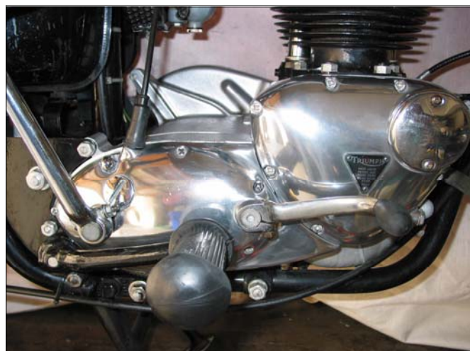
Same area after a ten minute session with a 3/8ths drill motor, a felt buff and some Mothers Aluminum Polish. Notice the transmission cover.
