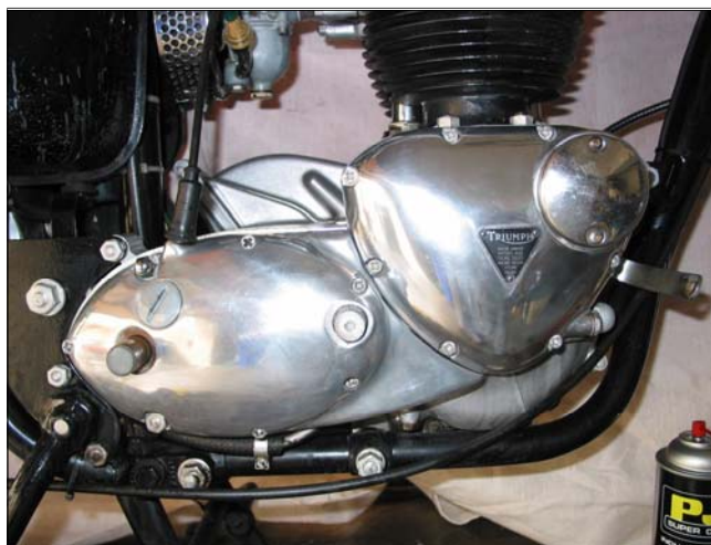
Timing and transmission outer cover prior to polishing. Shift lever, foot peg, exhaust, and kicker removed
