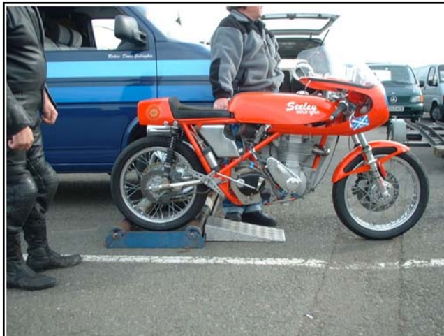
350cc Sealey Gold Star short-stroke 82X66. 34 BHP @ 8600RPM, lapped Isle of Man at 90.16 MPH. Oval flywheels increased revs 600 over circular wheels.
