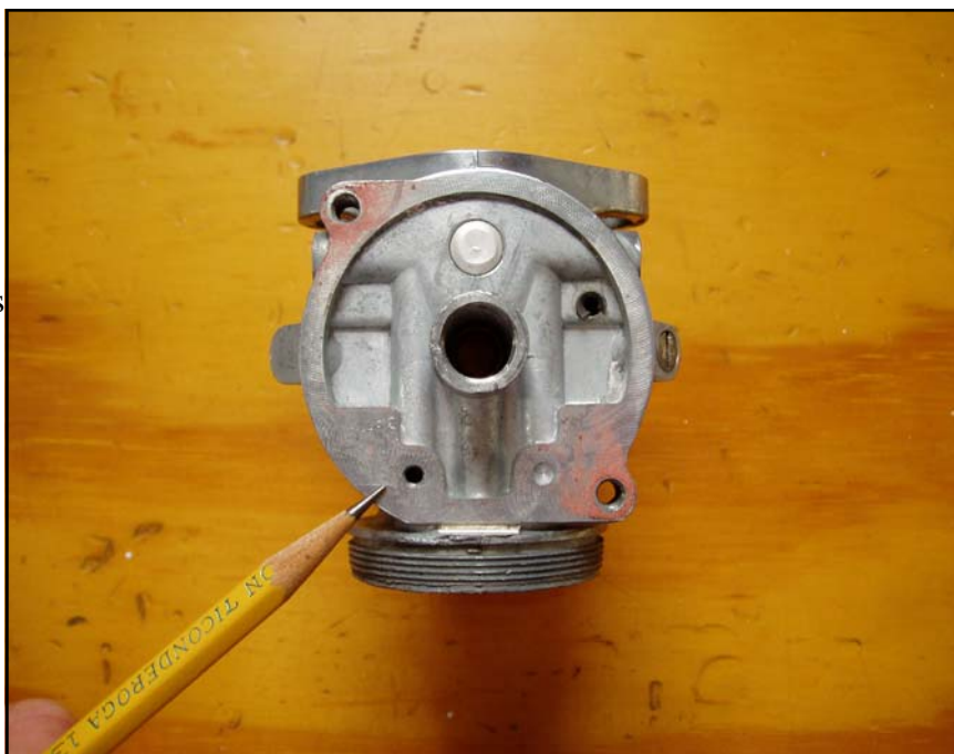
This Photo Shows The Underside Of An Amal Carburetor Body. The Pencil Points To The Pilot Jet Location And Pilot Air Passageway.
